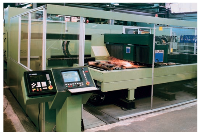
Laser cutting the steel plates.
