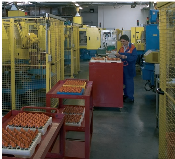
Loading the automated multi-axis CNC sharpening machines.
