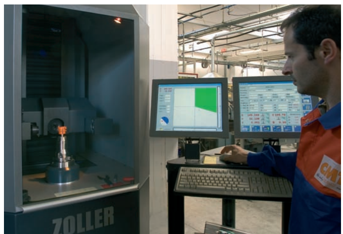
CMT's fully automatic measuring system.
