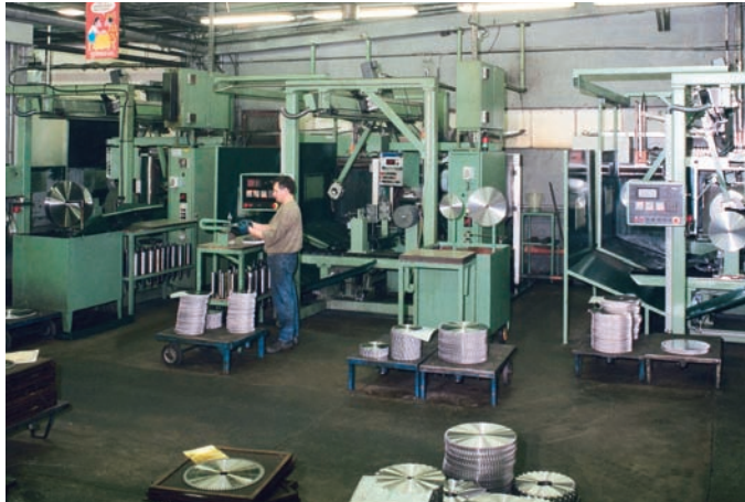
Grinding and tensioning the blades.
